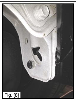
Step 7. Torque the (2) lower 3/8"-16x1-1/2" bolts to 25ft-lbs. Torque the top (2) 3/8"-16x5" bolts with nylon lock nuts until the lock nut makes firm contact with the bumper brace. Once the nut and bolt are firm, tighten nut an additional two turns.
